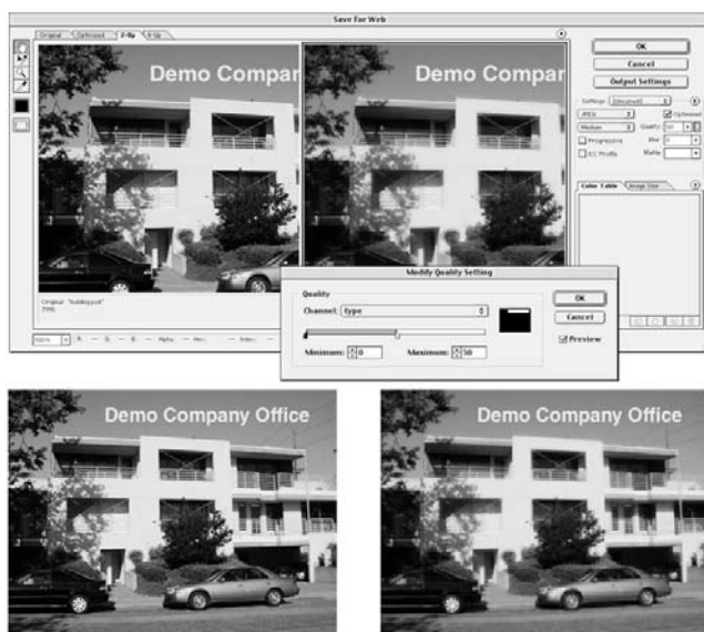
Figure 14-7. Distortions around flat color areas and text can be reduced with selective compression
